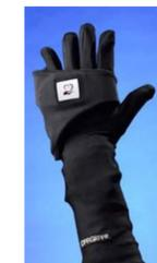
The electronic CPR glove, used for assisting medical staff into CPR procedure. (control frequency and depth of compressions)
