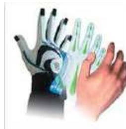
**Figure 3:** ShapeHand device use to produce 3D models of hands. (First person solution)
